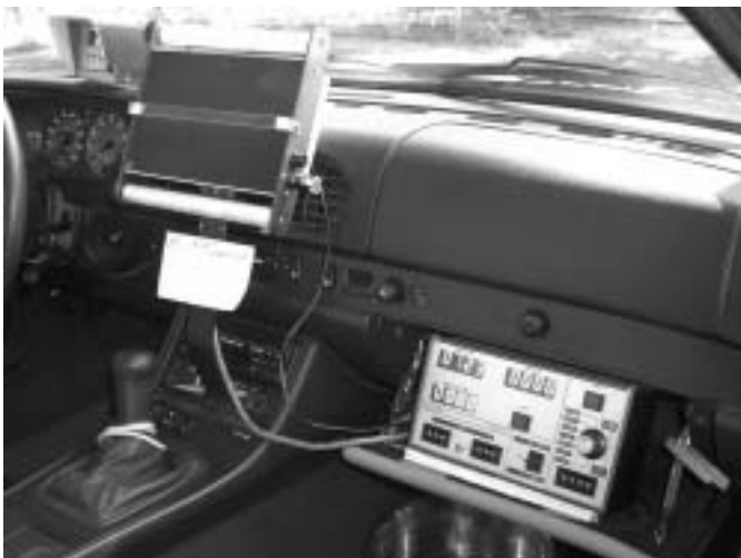
The cockpit of a "serious" rally car showing the navigator's computer and scroll holder for directions. This was not Rich and Mary Ann's Porsche!
