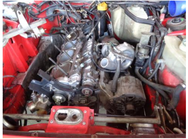
Long block in place
