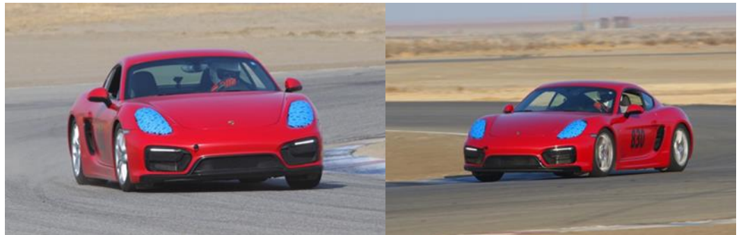
Cayman GTS in hard cornering – note the body roll as Jeff pushes his car
